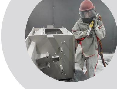
Our glass bead blasting service removes all impurities and deposits from steel surfaces to provide a smooth, uniform finish. Fine glass beads are applied to the surface at a low pressure avoiding any damage to the surface.
